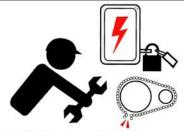
Do Not Perform Maintenance on Conveyor Until Electrical, Air, Hydraulic and Gravity Energy Sources Have Been Locked Out or Blocked
