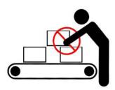
Do Not Load a Stopped Conveyor or Overload a Running Conveyor
